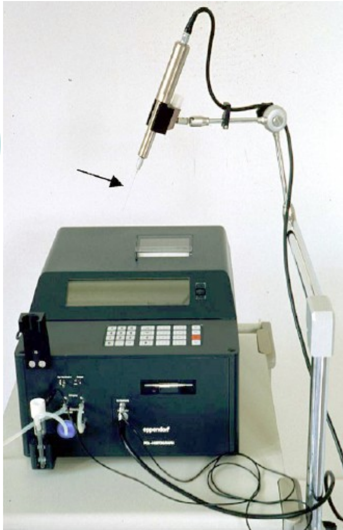
Polarographic fine needle probe
